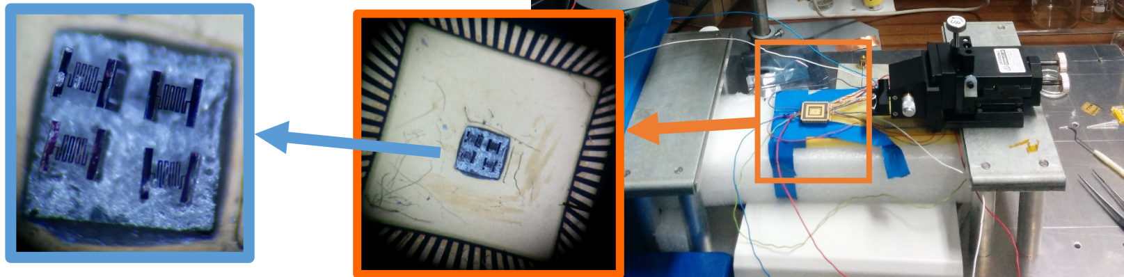
Fig. 7 - RFCMOS receiving circuit [2] and antenna array on top of Si die
